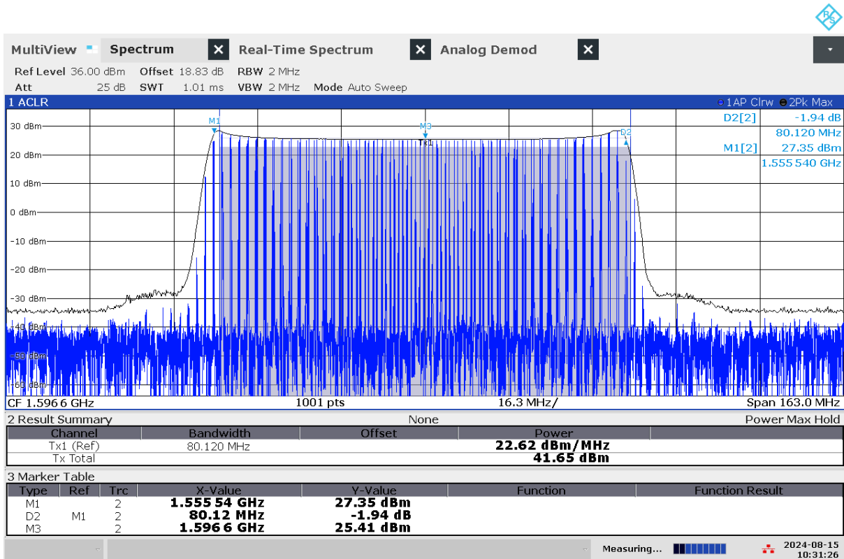
G 139: Frequency and power measurement of jammer H6.5 on antenna "5" (L1)
