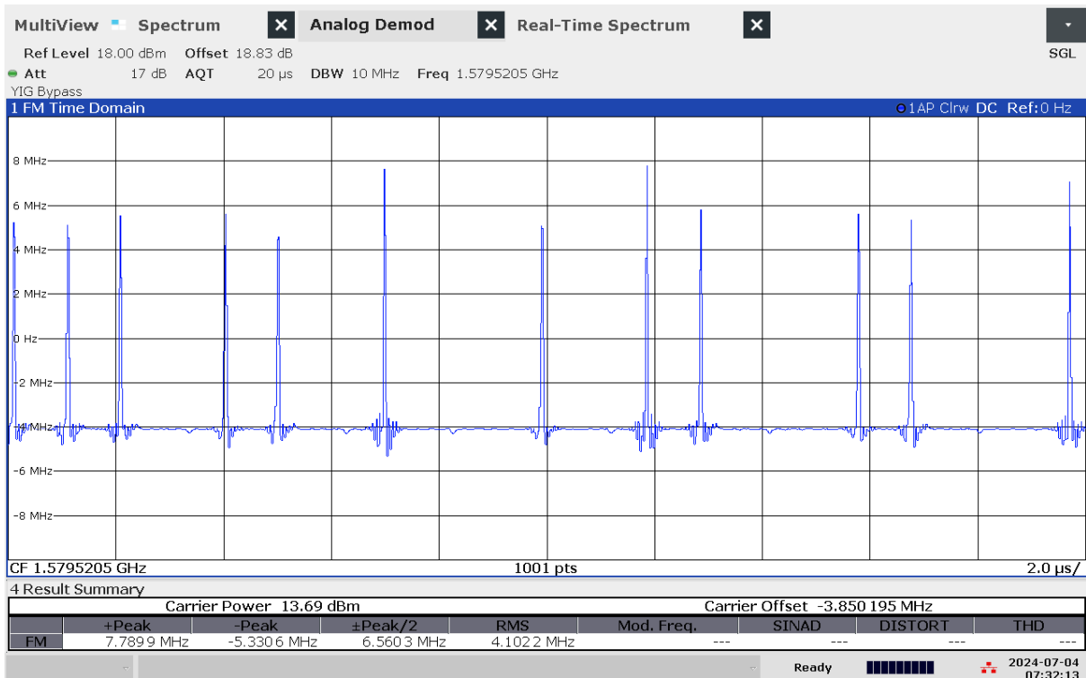
G 46: Time domain (analog demod) measurement of jammer H1.1 with antenna configuration L1 Narrow band High Power (NB HIGH PWR)
