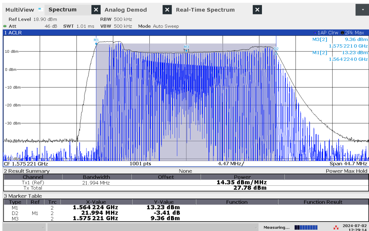
G 64: Frequency and power measurement of jammer H1.2
