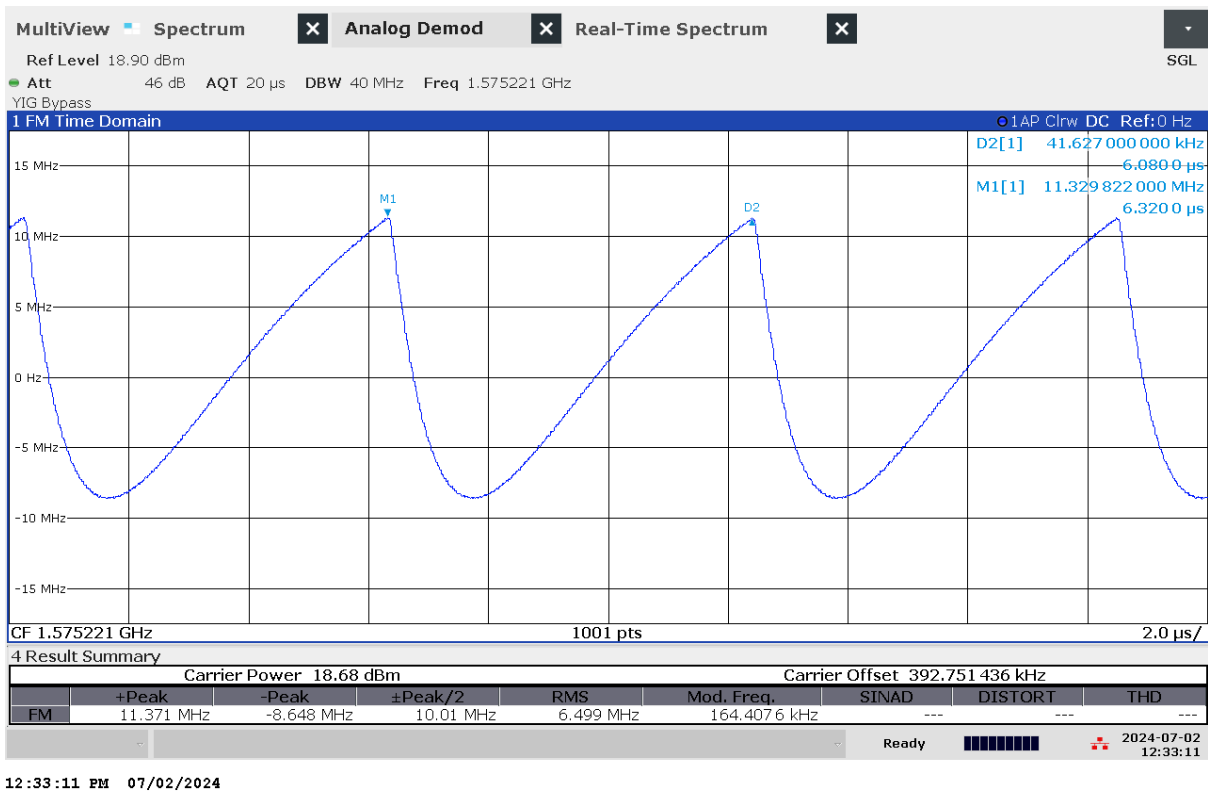
G 66: Time domain (analog demod) measurement of jammer H1.2
