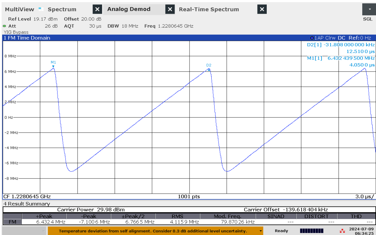
G 82: Time domain (analog demod) measurement of jammer H3.3 on antenna "medium" (L2)
