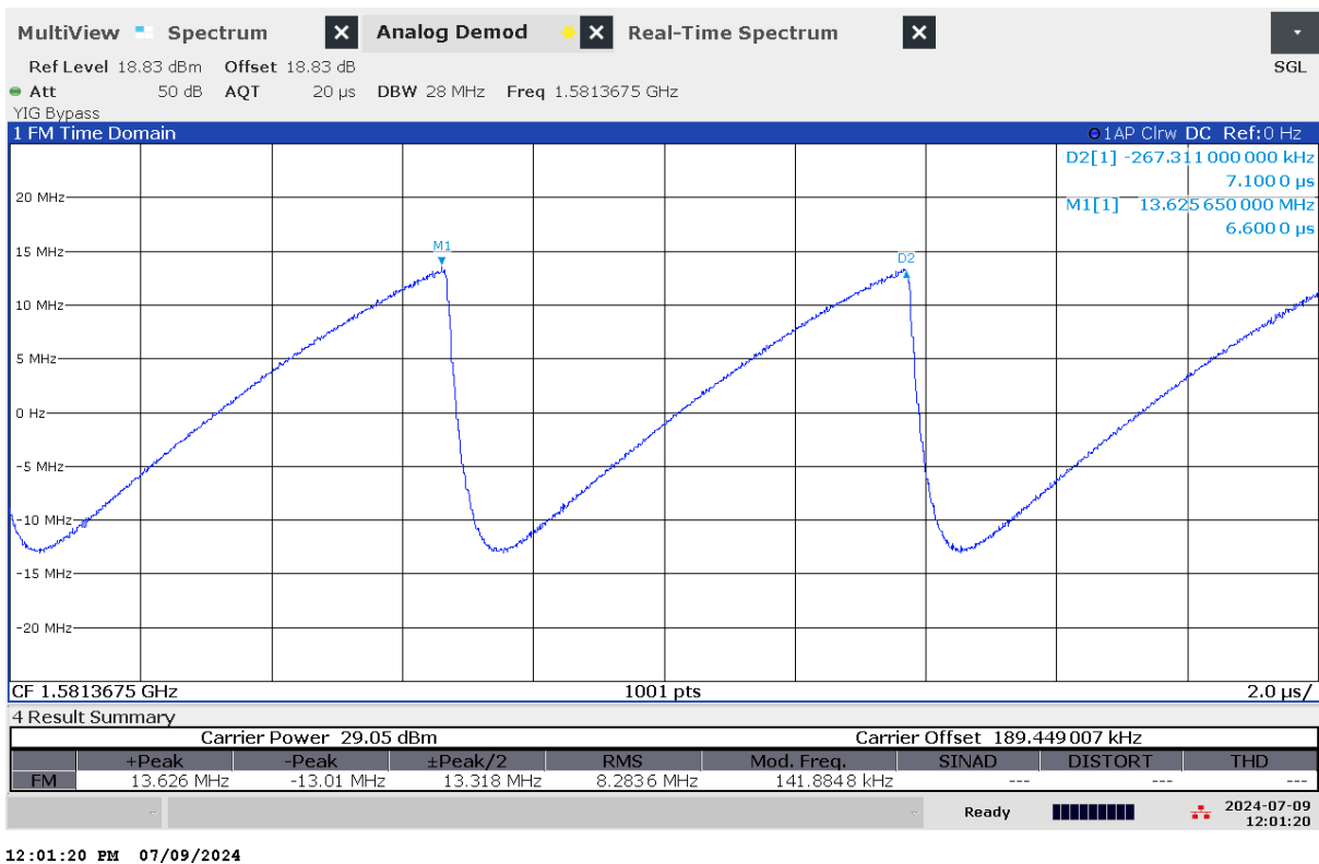
G 124: Time domain (analog demod) measurement of jammer H6.3 on antenna "4" (L1)
