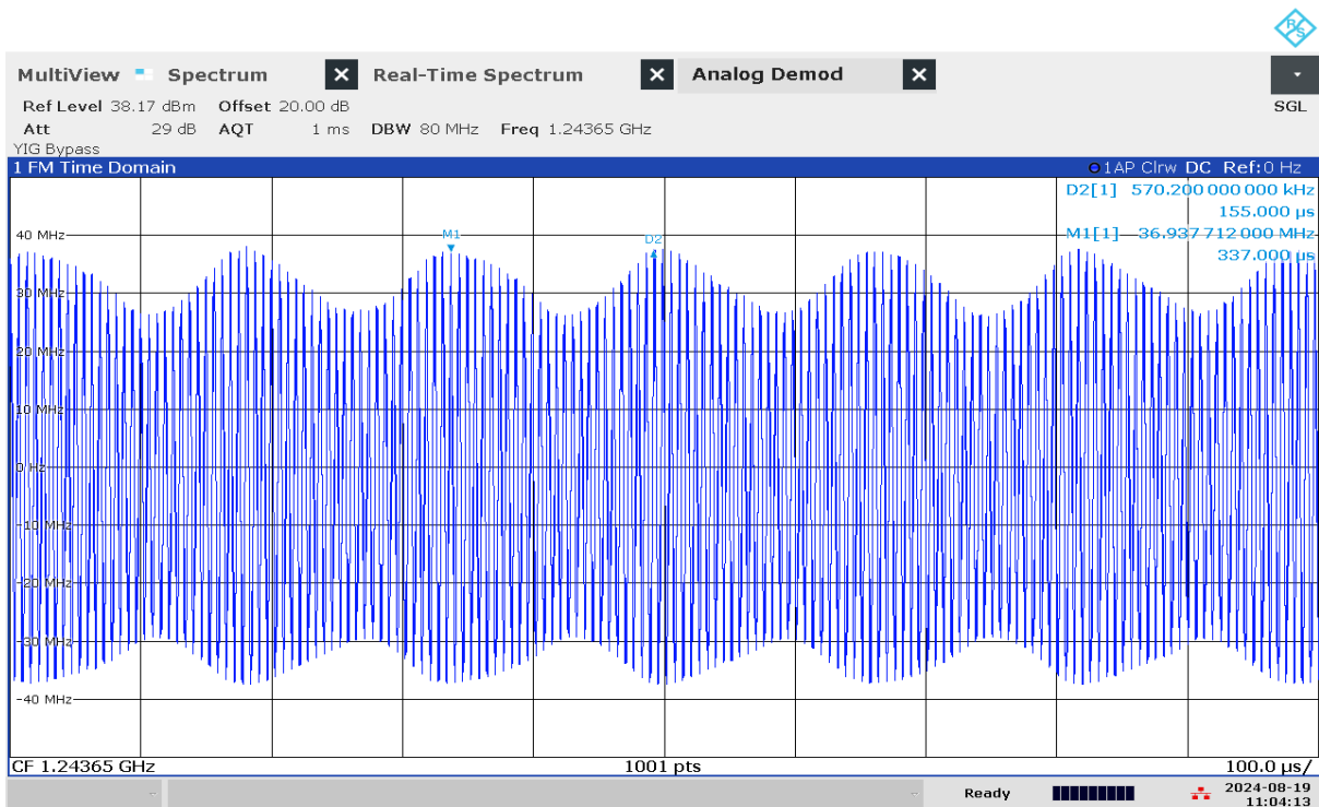
G 167: Time domain (analog demod) measurement of jammer F6.1 on antenna "F4" (L2)
