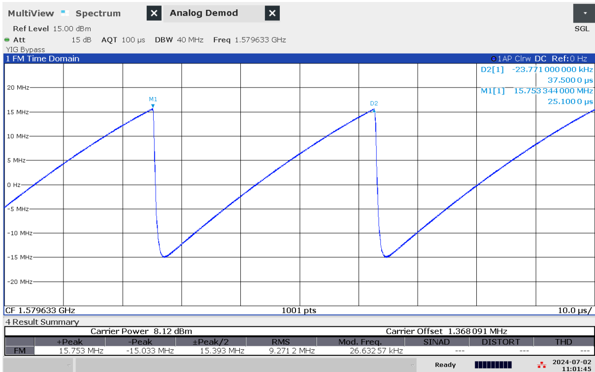
G 9: Time domain (analog demod) measurement of jammer S1.3
