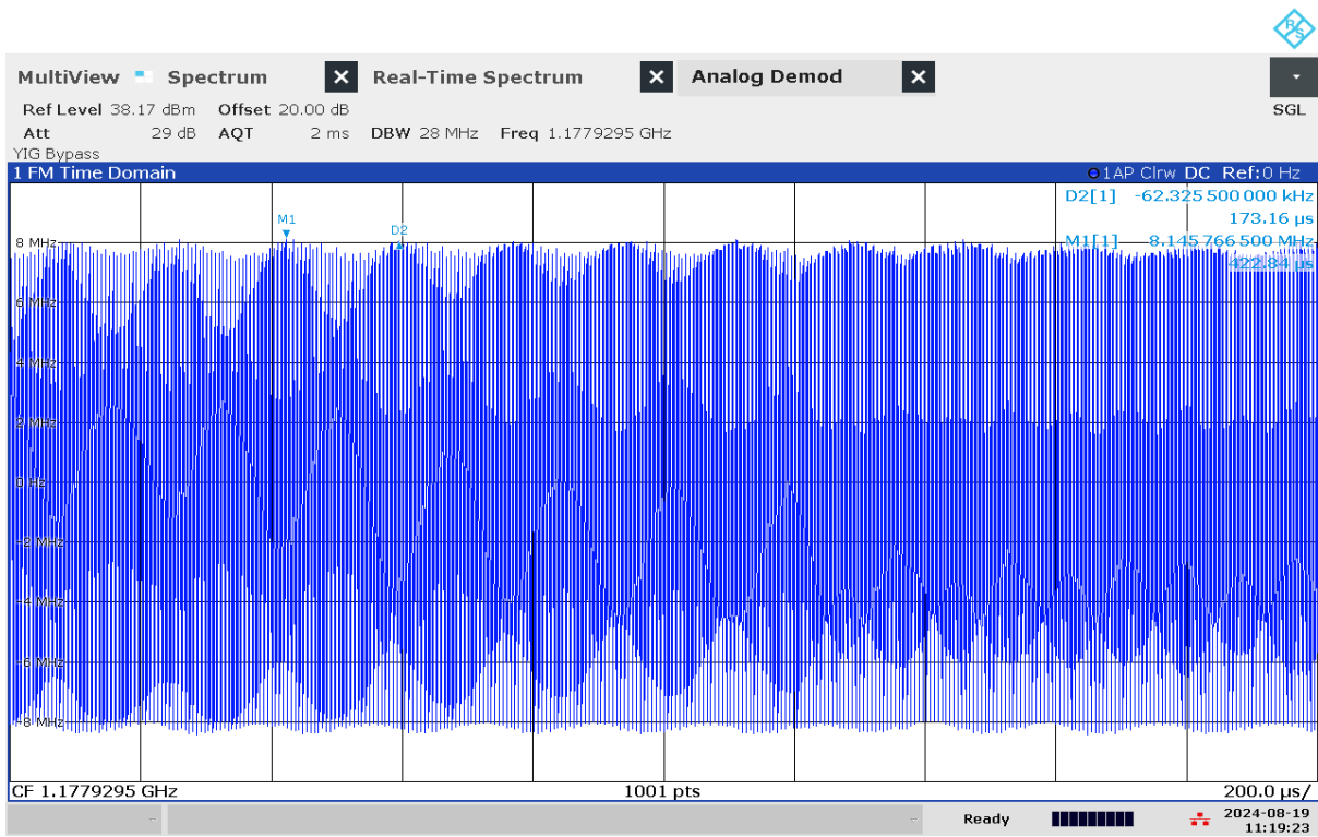
G 170: Time domain (analog demod) measurement with wider span of jammer F6.1 on antenna "F6" (L5)
