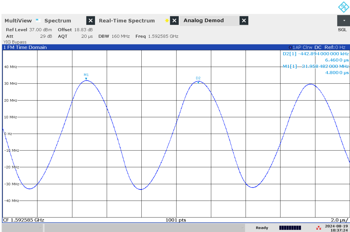
G 163: Time domain (analog demod) measurement of jammer F6.1 on antenna "F2" (L1)
