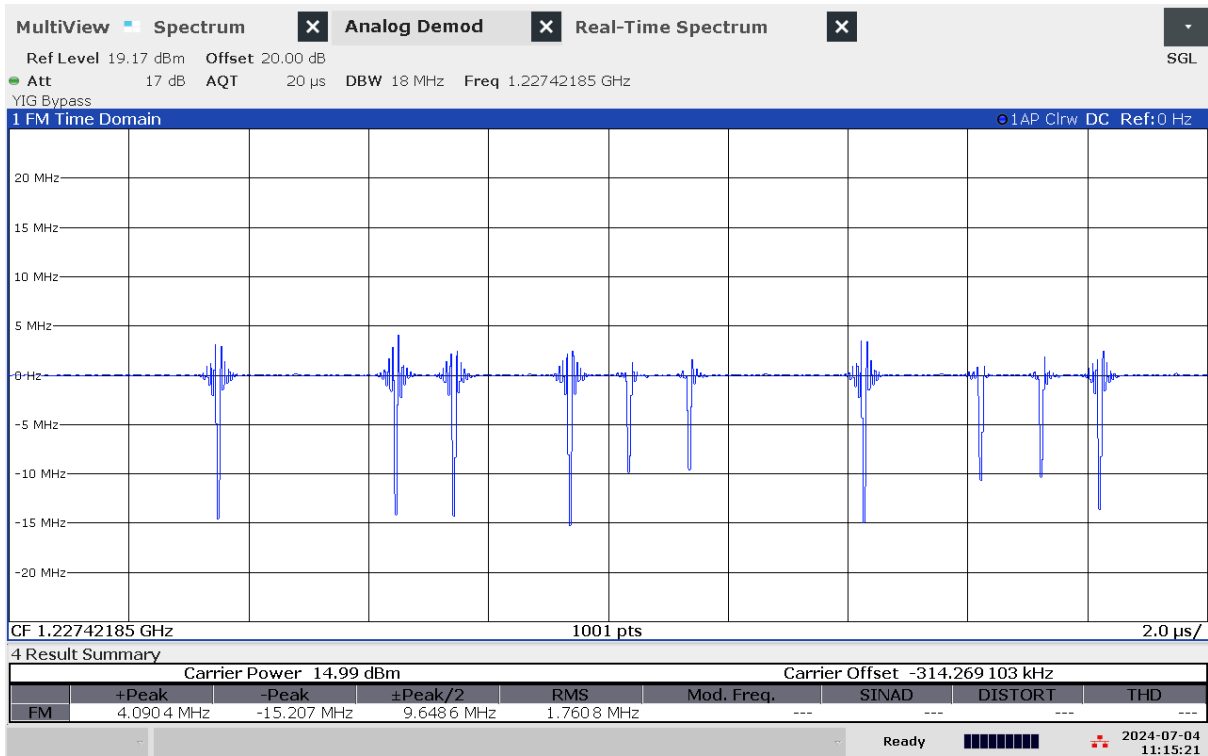
G 60: Time domain (analog demod) measurement of jammer H1.1 with antenna configuration L2 Narrow band High Power (NB HIGH PWR)
