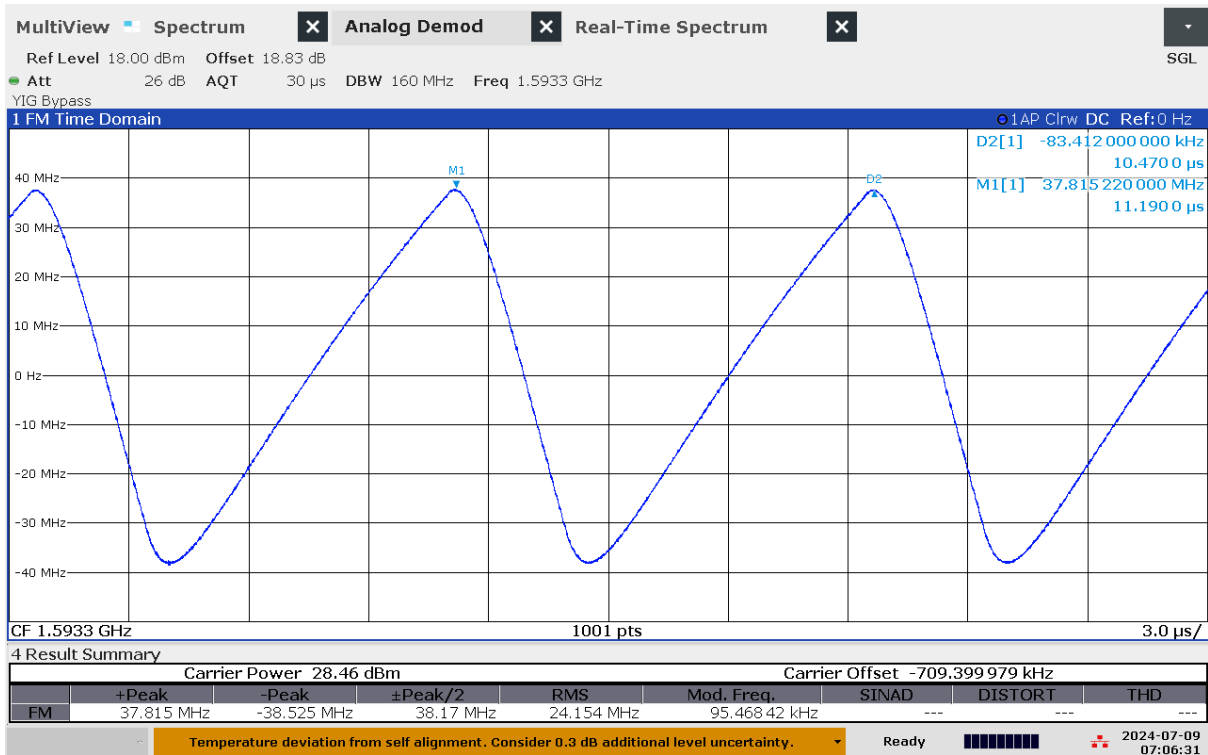
G 173: Time domain (analog demod) measurement of jammer H8.1 on antenna "6"
