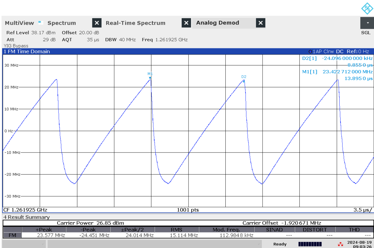
G 96: Time domain (analog demod) measurement of jammer H4.1 on antenna "1" (L1)
