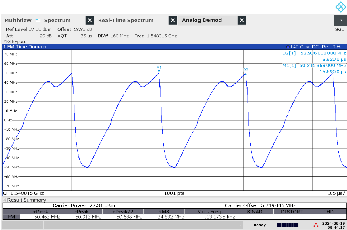
G 96: Time domain (analog demod) measurement of jammer H4.1 on antenna "1" (L1)
