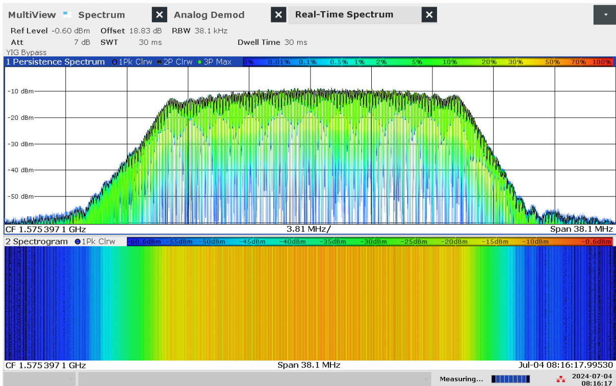
G 45: Real-time persistence and spectrogram measurement of jammer H1.1 with antenna configuration L1 Chirp High Power (CHIRP HIGH PWR)
