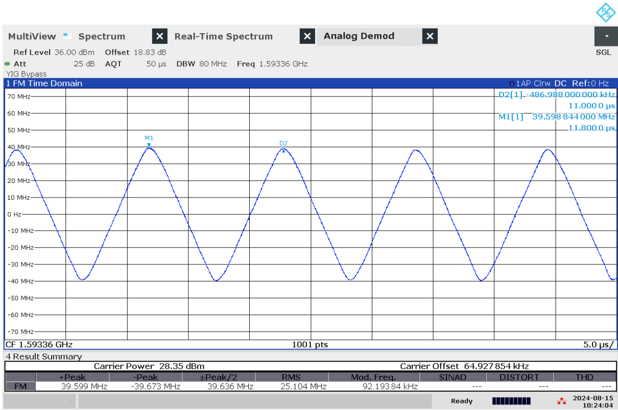
G 136: Time domain (analog demod) measurement of jammer H6.4 on antenna "5" (L1)
