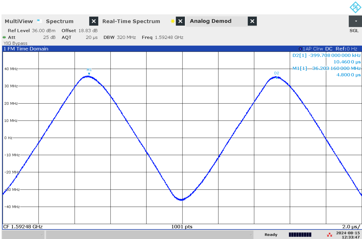
G 154: Time domain (analog demod) measurement of jammer H6.6 on antenna "5" (L1)
